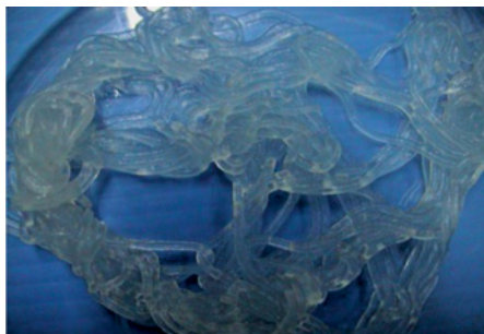
Plate 12.16 Cooked clear glass noodle made from edible canna starch (Japanese Green) using a laboratory single screw with feed moisture content at 30%, barrel temperature of zone 1: 2: 3 at 70: 70: 100 °C, feeder and screw speed at 50 rpm and 30 rpm respectively
